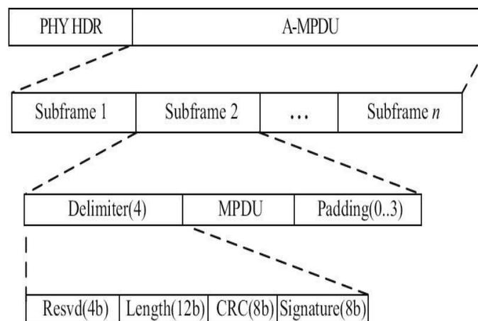
Figure 1: A-MPDU Aggregation in 802.11n
