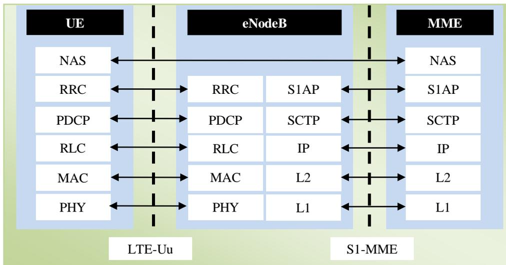
Fig. 4 Control plane protocol stacks for EPS in LTE architecture
