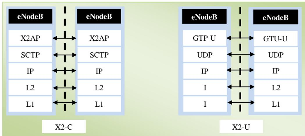
Fig. 3 Control and user plane protocol stacks for x2 interface in LTE Architecture
