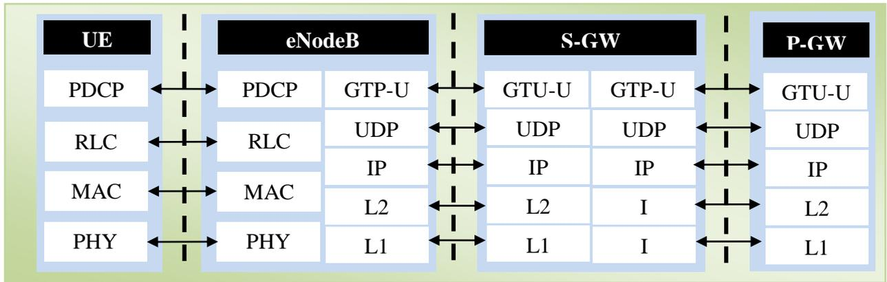
Fig. 2 User Plan Protocol Stack EPS in LTE interface
