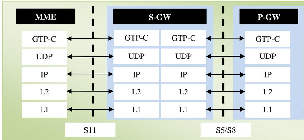
Fig. 5 User plane protocol stacks for EPS in LTE architecture.
