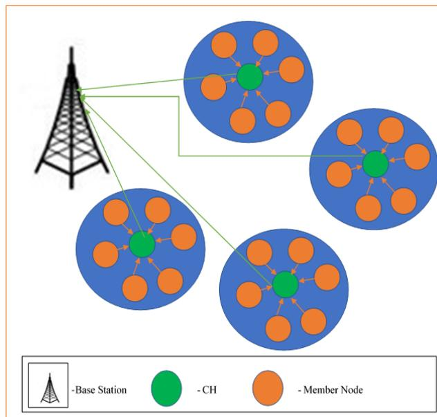
Figure 1.communication structure of WSN
