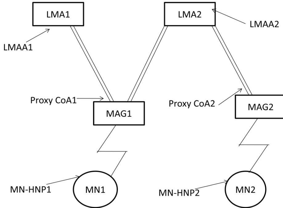
Figure 1: Proxy Mobile IPv6 Domain
