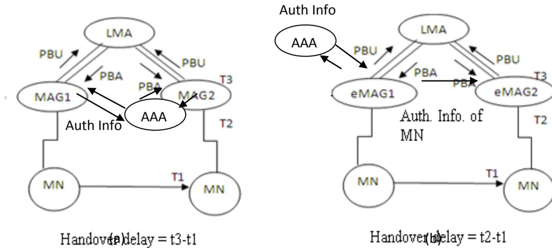
**Figure 3: Comparison of working of MAG and eMAG**
