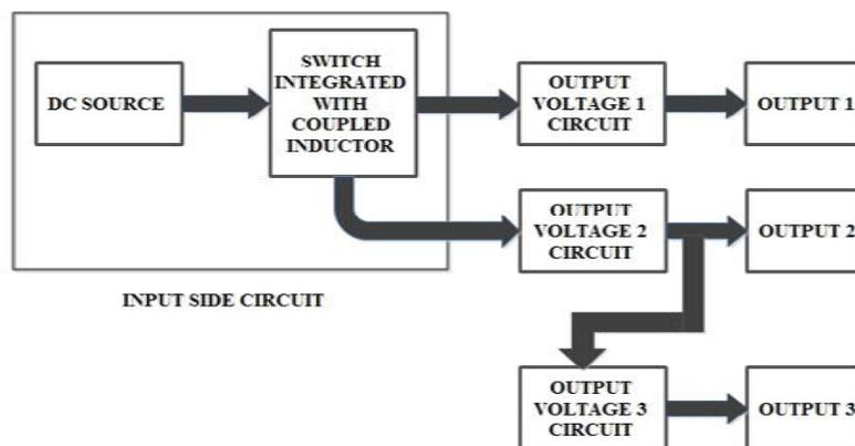
Fig.1 Proposed Single Input Multiple Output dc-dc converter Block Diagram
