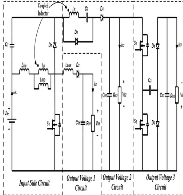
Fig.2 Proposed Single Input Multiple Output dc-dc converter Circuit Diagram
