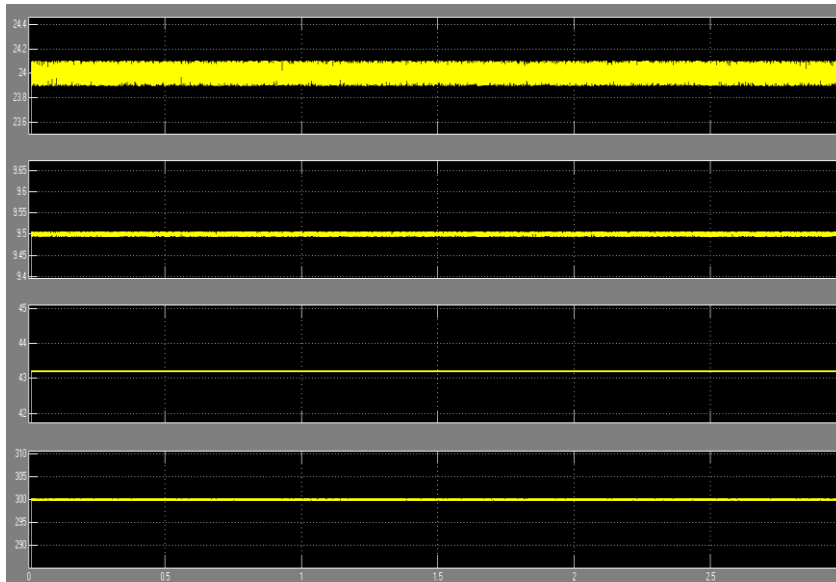
Fig 7.voltage and current responses of proposed converter with 200-W output power
