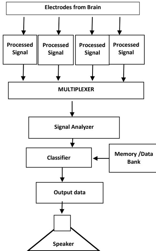
Fig.3: Schematic diagram [working of proposed methodology]
