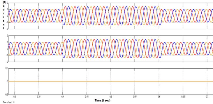
**Figure .7 Current Waveforms Under Overload Condition**
