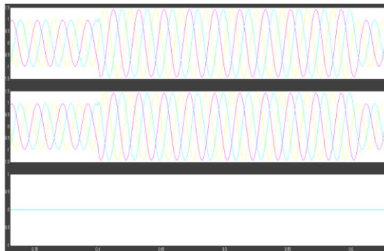
**Figure .10 Current Waveforms Under Overload Condition**
