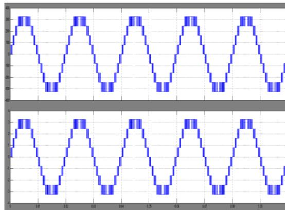
**Figure.9 Nine Level Output Voltages and Currents**
