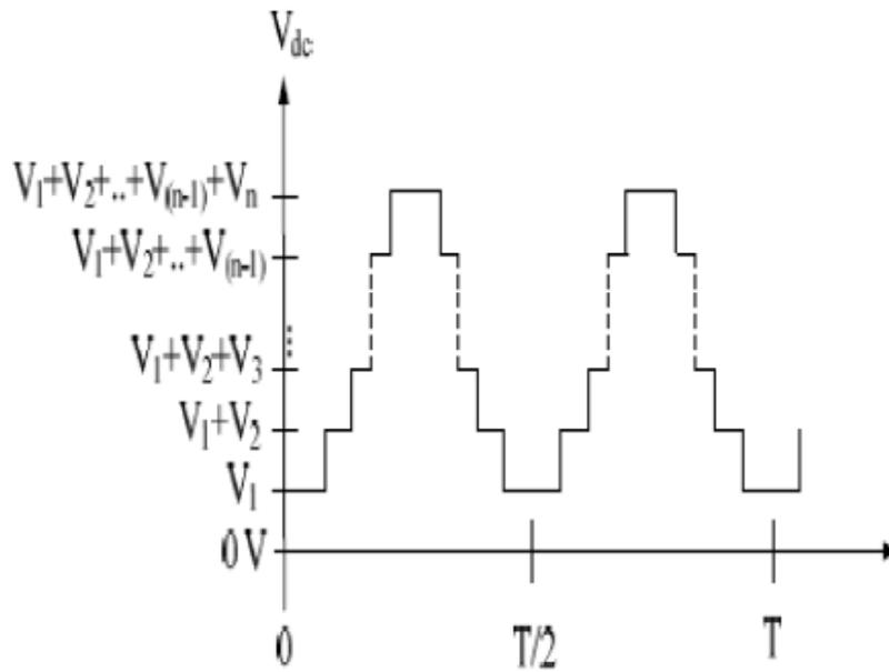
Figure.2 Typical output waveform of Vdc
