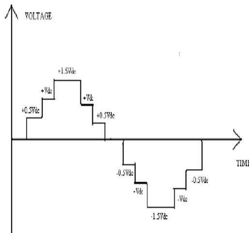
Figure.4 the seven level output voltage produced by the conventional inverter
