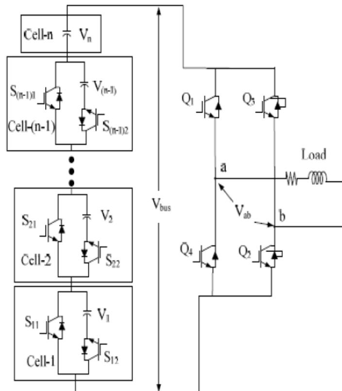
**Figure.1 Structure of the conventional cascaded dc link MLI** The above figure shows Structure of the conventional cascaded dc link MLI
