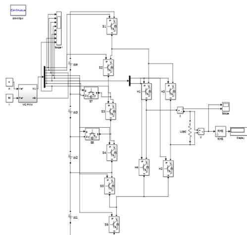
Figure.7 Simulation of Proposed Nine-Level Inverter
