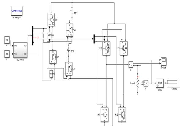
Figure.6 Simulation of Conventional Seven-Level Inverter
