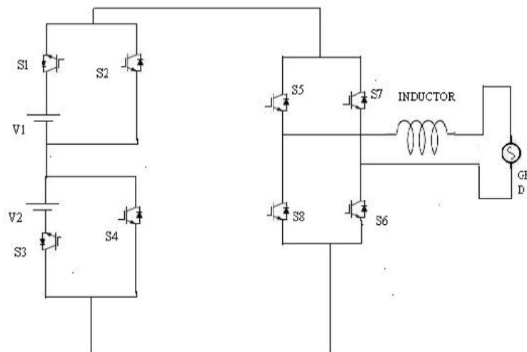
Figure.3 Conventional single-phase seven-level inverter with less number of power elements for grid connection
