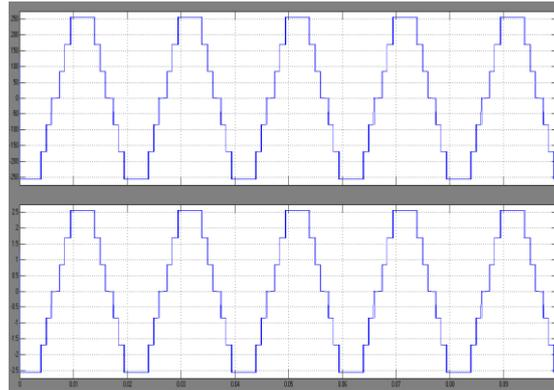
**Figure.8 Seven Level Output Voltages and Currents**
