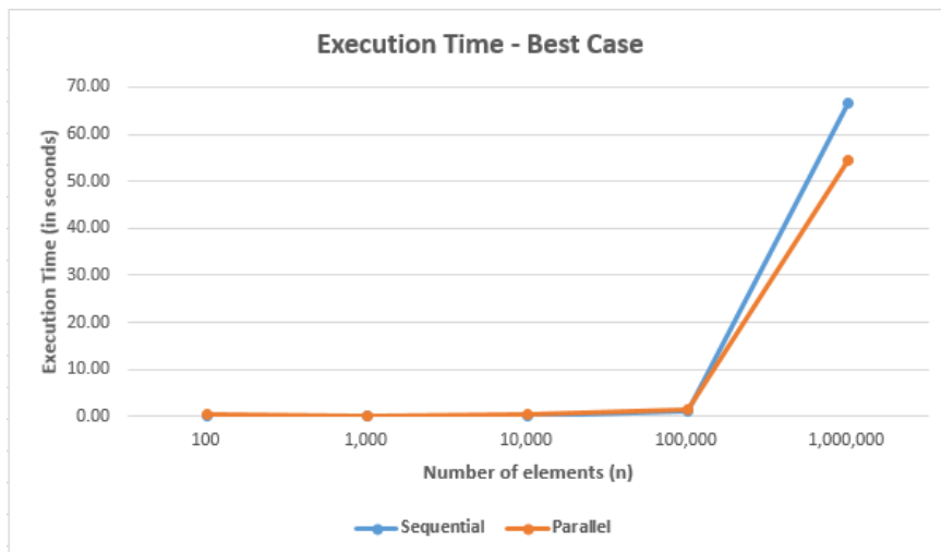
Fig. 3 Performance Comparison of Sequential and Parallel Merge Sort (Best Case)
