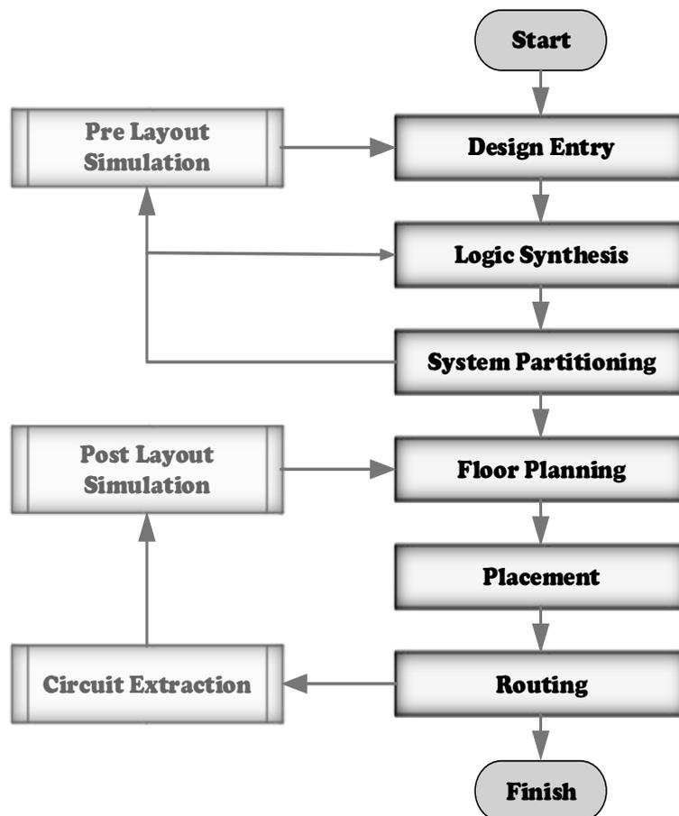
Figure 2: ASIC Physical Design Flow
