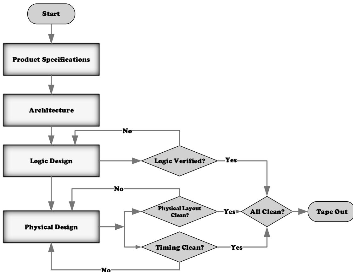
Figure 1: ASIC Design and Implementation Flow
