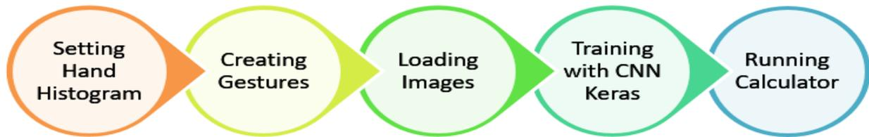
Fig. 4 Process of Hand Gesture Recognition
