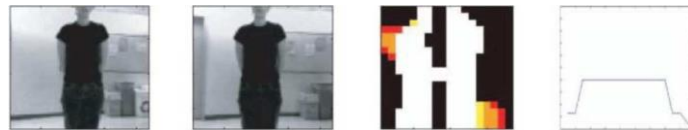
Fig.3 Example of TVS operation: image from the two camera, disparity map, and the corresponding signals sent to the tacto belt.
