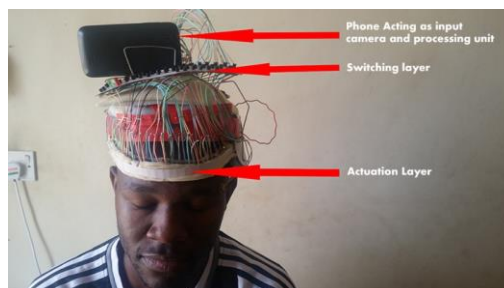
Fig. 11 Annotated headset, part the control unit is a circuit behind the phone
