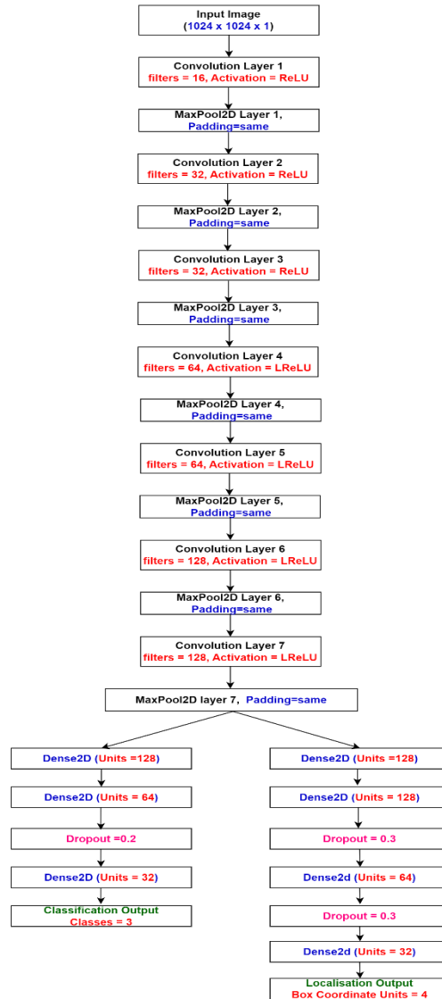
Fig. 4. The Proposed Multi-Output Deep CNN Model
