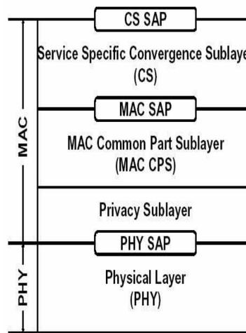
Fig. 1: WiMAX physical and MAC layer architecture
