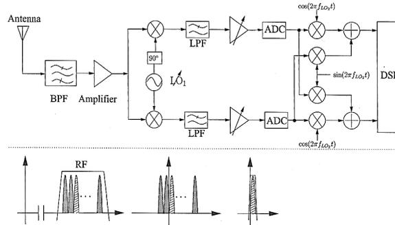
Figure 1.4: Low-IF receiver architecture
