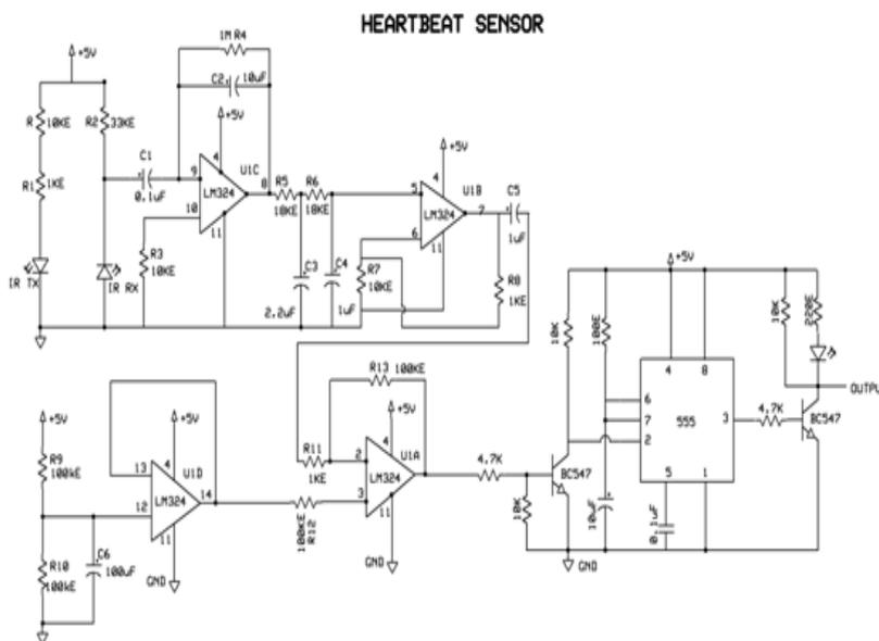
Fig 16: Circuit Diagram of Heartbeat Sensor
