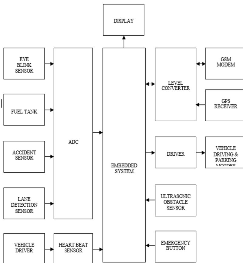
Fig. 1: Block diagram of Vehicle tracking and locking system based on GSM and GPS
