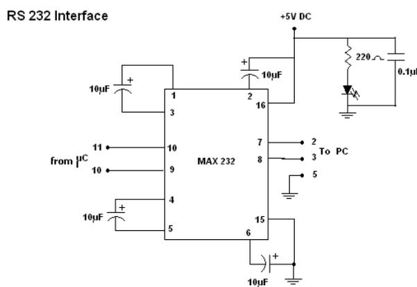
Fig 17: RS232 Level Converter
