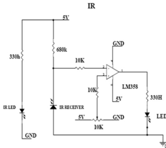
Fig 6: IR Sensing Circuit
