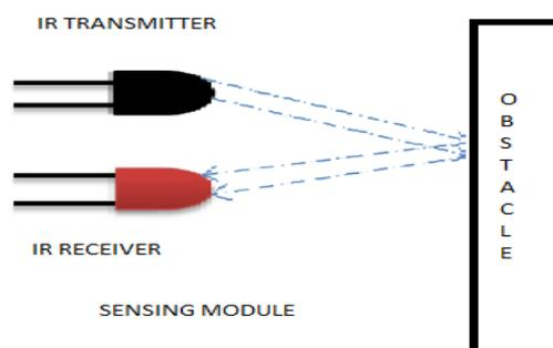
Fig 7: obstacle sensing module
