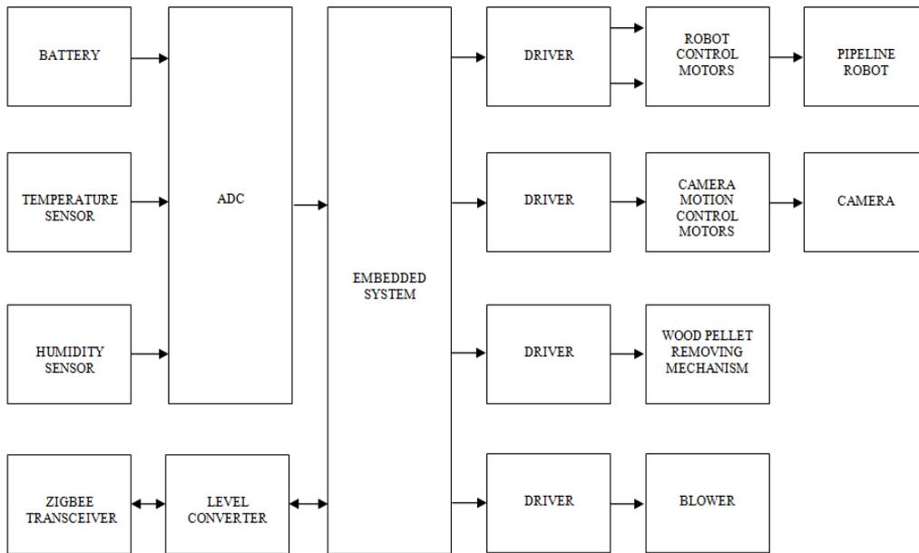
Fig. 1: Block diagram for robo section
