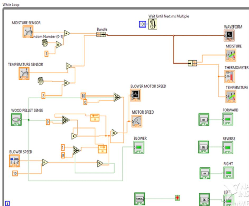
Fig 6: Block panel of simulation
