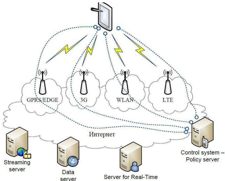
Fig.3 Functional Architecture for 5G Mobile Networks
