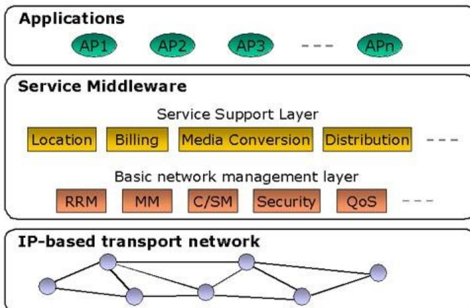
Fig.1 Layered view of the IP-based Core Network in 4G
