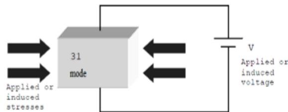
**Figure 4** 3-1 Mode of electromechanical coupling [1]
