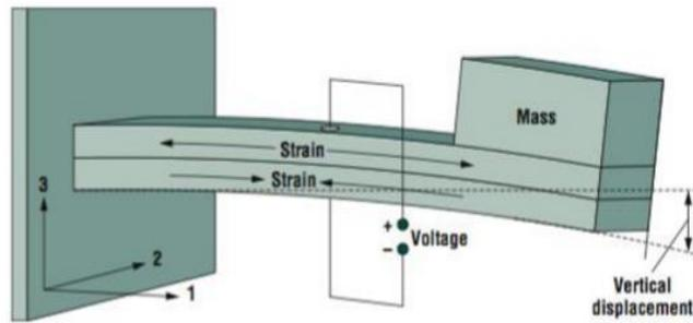
**Figure 3** Strain is generated along the length of the beam (by 3-1 mode) [2]
