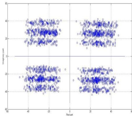
**Fig.12- Constellation diagram for multi-path case 1**
