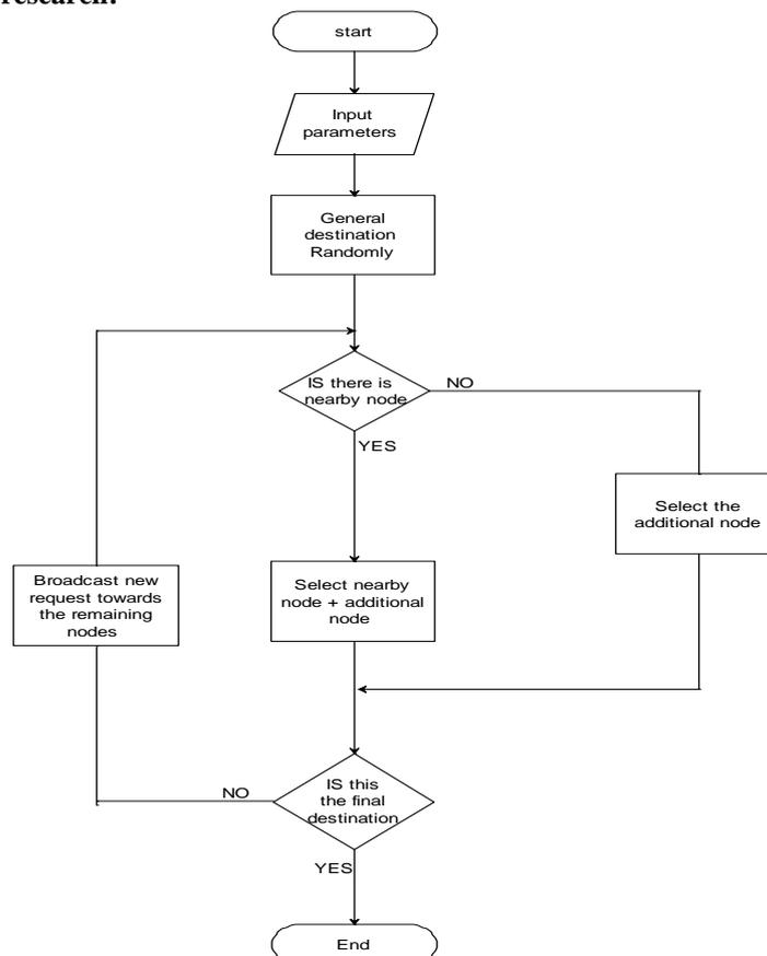
Fig. 4 flowchart of evaluating routing protocols (AODV, AOMDV, DSR)
