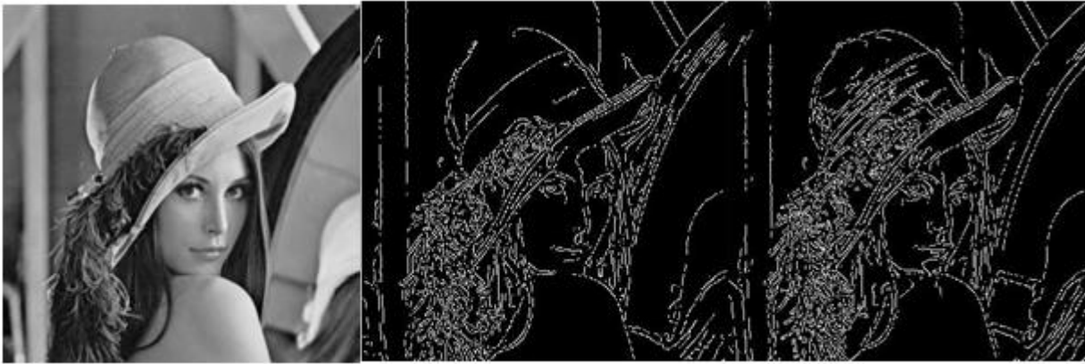
Figure8. Simulation Results, Middle Image (the Proposed Method), the Right One Is Canny Edge Detection
