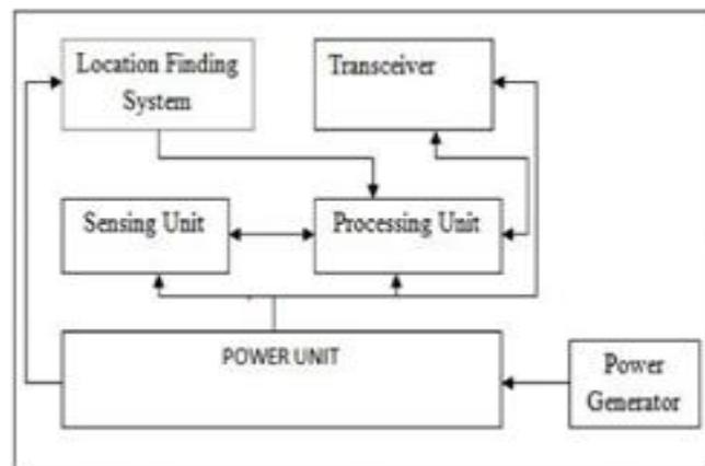
Fig. 1 Architecture of wireless sensor node [5]
