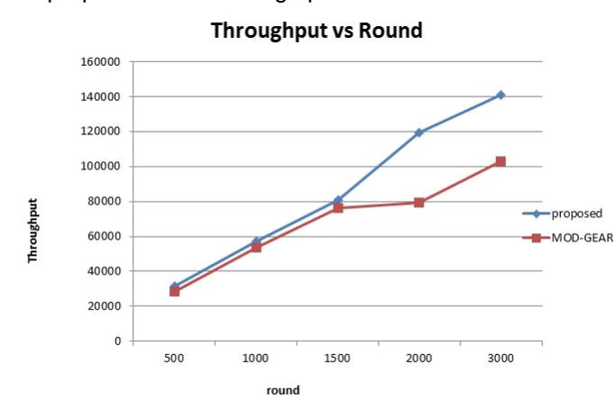
Fig. 4. comparison of average throughput MOD-GEAR and PROPOSED delivery ratio the proposed work has higher than Modified Geographical Energy-Aware Routing Protocol.
