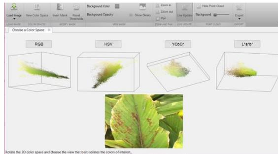
Figure 5: Sample Color Segmentation for Viral Leaf Spot
